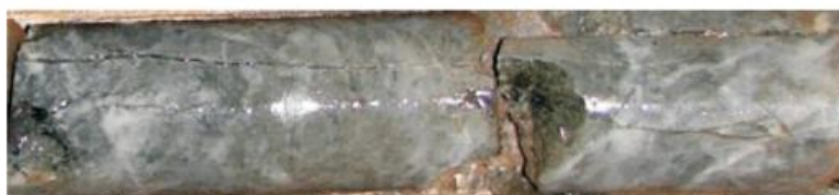
Intense silicified zone with disseminated Molybdenum at 1647 feet.
