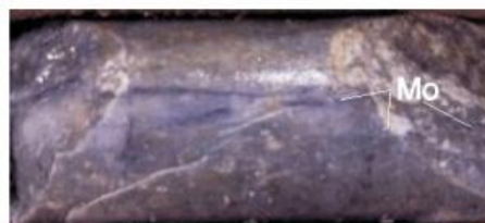
Molybdenum (Mo) bearing veins at 1462 feet .
