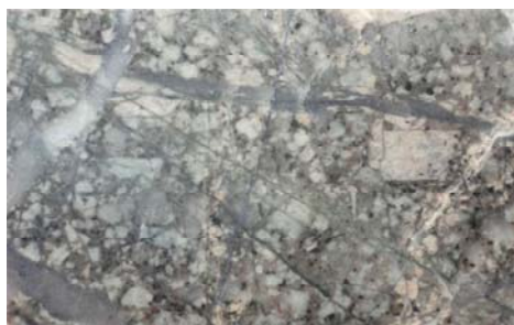
a) Quartz - MoS2 veinlets in porphyry unit Tbqmp3 C35-08 (2291 ft)
