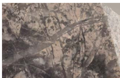
b) Stockwork Quartz - MoS2 veinlets in Quartz Monzonite unit Kqm C35-08 (2496 ft)
