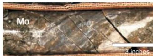
Excellent Molybdenum (Mo) bearing veins at 722 feet
