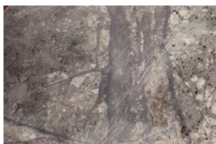
c) Quartz MoS2 veinlet in intrusive breccia unit Tbx C08-37 1896.5 ft
