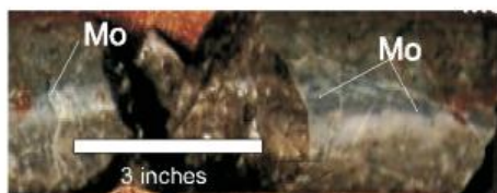
Quartz stockwork with Molybdenum (Mo) at 298 feet
